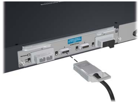
Figure 2-11. Connecting copper cable.
